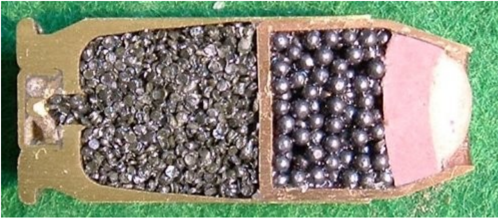
.45 ACP with eraser and nickered case is headstamped R-P 45 AUTO
